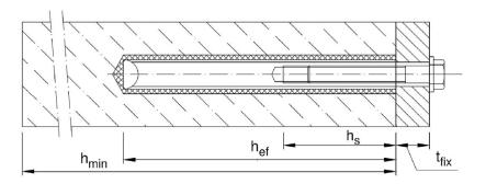
$t_{fix}$  = thickness of fixture
